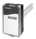
The Carbon Dioxide (CO<sub>2</sub>) Sensors and Controllers are standalone carbon dioxide (CO<sub>2</sub>) sensors for use in determining ventilation necessity with HVAC controllers. The sensor measures the CO2 concentration in the ventilated space or duct. The sensors are used in ventilation and air conditioning systems to control the amount of fresh outdoor air supplied to maintain acceptable levels of  ${\rm CO_2}$  in the space.
